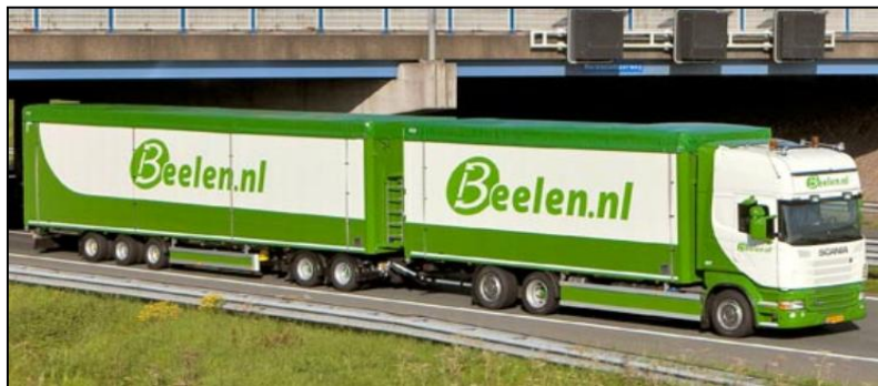
Fig. 5: EMS – weight-oriented variant
